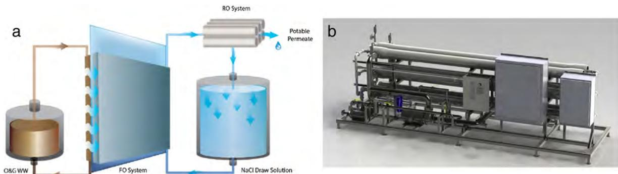
**Fig. 4.** HTI's second generation Green Machine. (a) The FO treatment system operates under constant influent draw solution concentration using an RO membrane reconcentration system. (b) 8-inch spiral wound FO elements are housed in membrane pressure vessels and are installed on a trailer tested at O&G drilling locations in the field.
