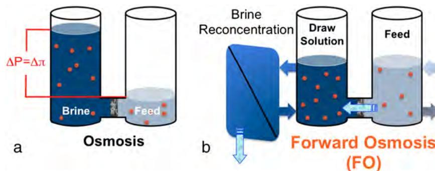
**Fig. 1.** A synthetic polymeric membrane separates a feed stream and a concentrated draw solution, and the osmotic pressure difference across the membrane facilitates diffusion of water through the membrane: (a) the osmosis process and (b) FO process when the osmosis process is coupled with a brine reconcentration system, producing high quality product water, while reconcentrating the FO draw solution to maintain constant osmotic pressure.
