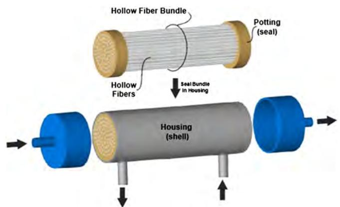
**Fig. 11.** Hollow fiber FO membranes are group in bundles of varying size and potted at each end. The potted membrane bundle is then installed into a membrane housing or shell where, depending on the membrane orientation, the draw solution can either flow on the inside or outside of the hollow fiber.
