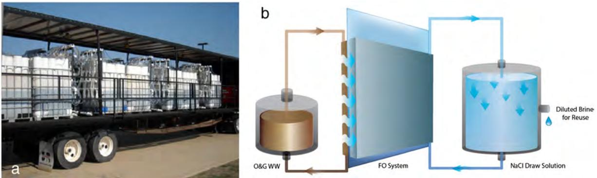
**Fig. 3.** (a) The HTI's first generation Green Machine mobile system. (b) The FO treatment system operated under osmotic dilution using 20–280 vertically oriented spiral wound FO elements. The membrane elements were grouped into several pods and were installed on a trailer (b) that was operated at O&G drilling locations in the field.
