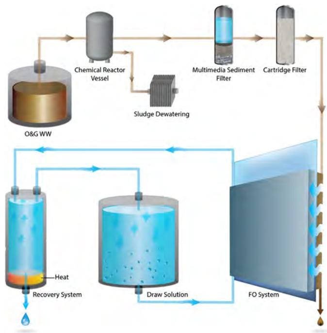
**Fig. 5.** Oasys Water's Membrane Brine Concentrator. The FO treatment system operates under constant influent draw solution concentration using a thermolytic reconcentration system. Several pretreatment technologies are used prior to FO membrane treatment to reduce oil emulsions and elevated hardness concentrations in O&G wastewaters.
